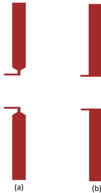
Figure 3.9 – Tapered (a) and Non-Tapered (b) Slot.
