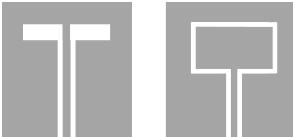
Figure 5.1 - Slot Antenna (a) and Loop Antenna (b).
